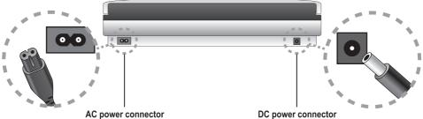
When connecting to AC 100-240V power outlets at home, the AC power cable is to be connected to the rear AC socket of the appliance.
